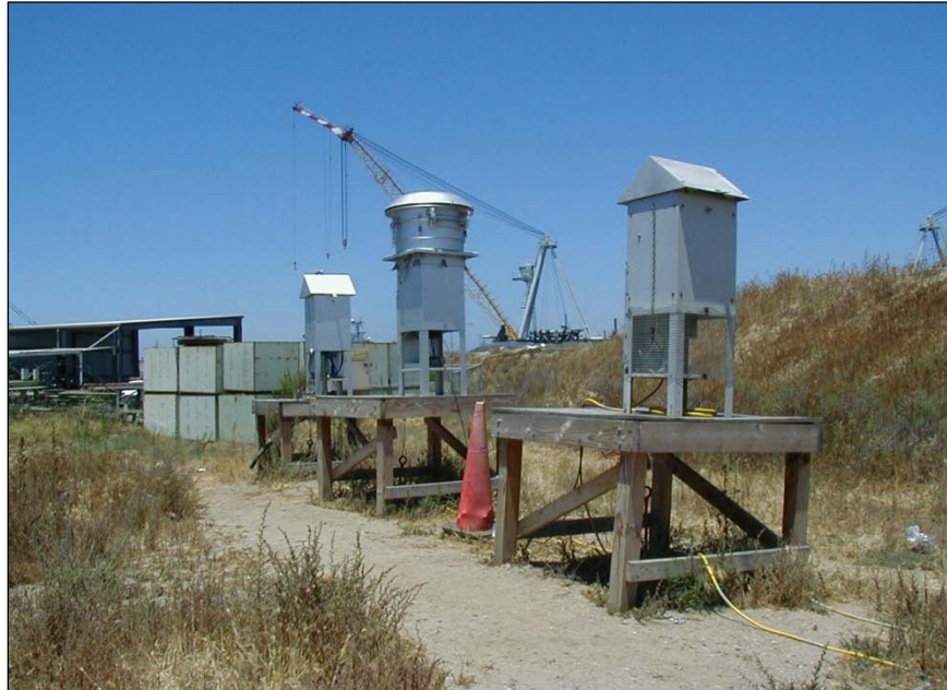
Figure 3-1: Example High Volume Sampler Installation
