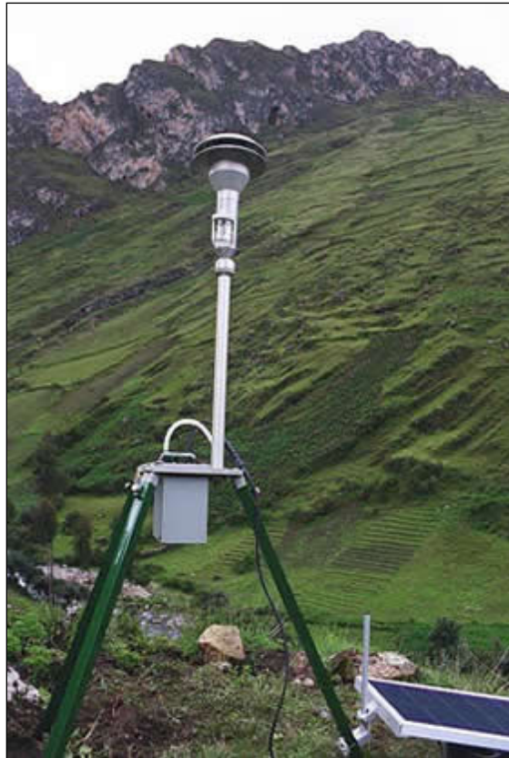
Figure 3-2: Example High Volume Sampler Installation
