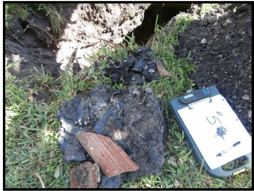
Test Pit 5. Burnt material, clay and dark residue.
