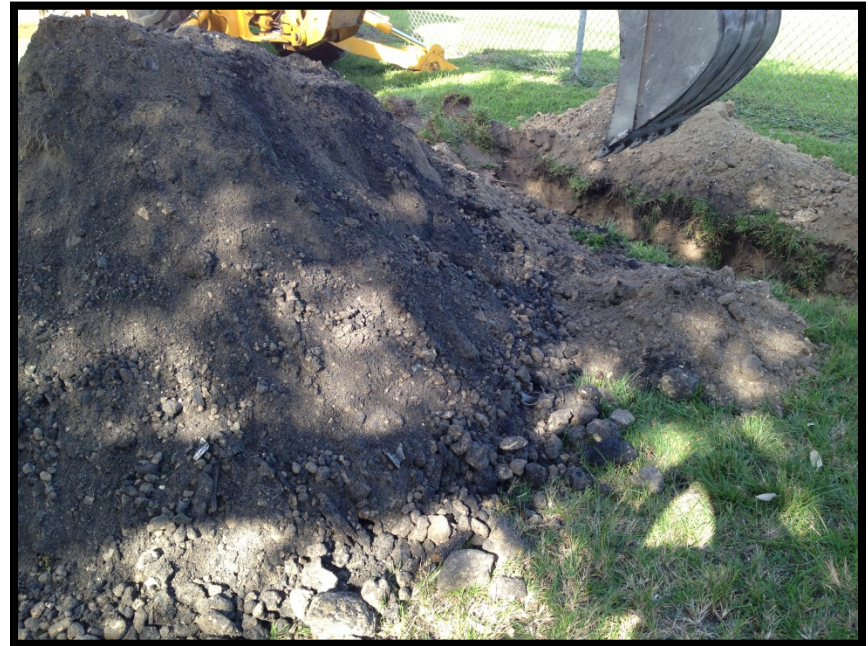
Test Pit 15. C+D debris with black residue
