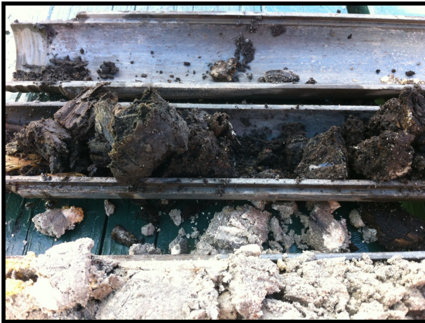
SB 16. Rusted metal pieces mixed with soil (top split spoon).
