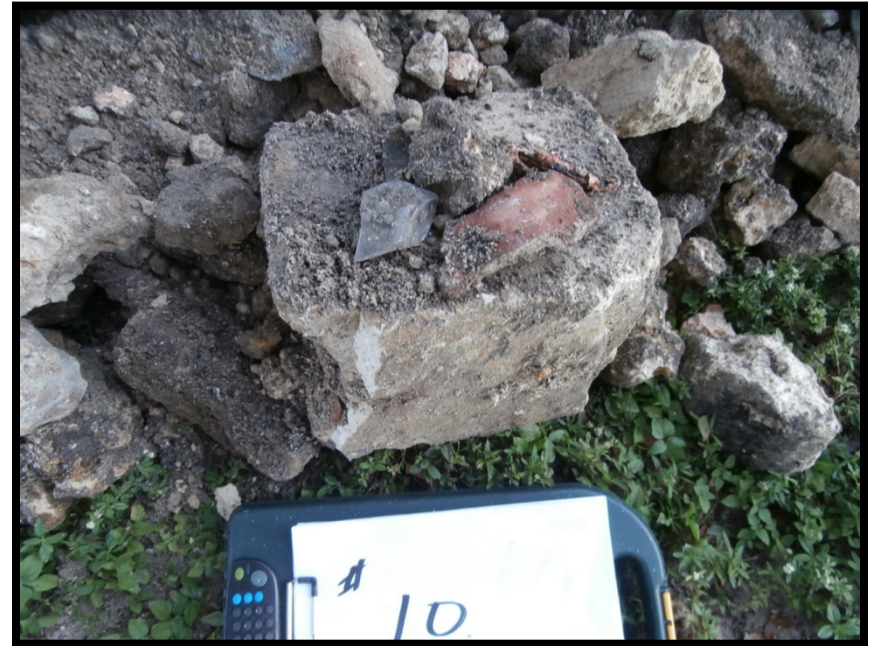
Test Pit 10. Broken glass and C+D debris.
