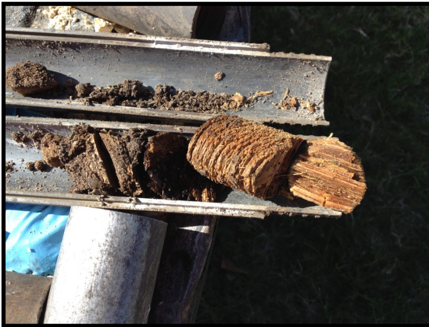
SB 13. Processed wood pieces.
