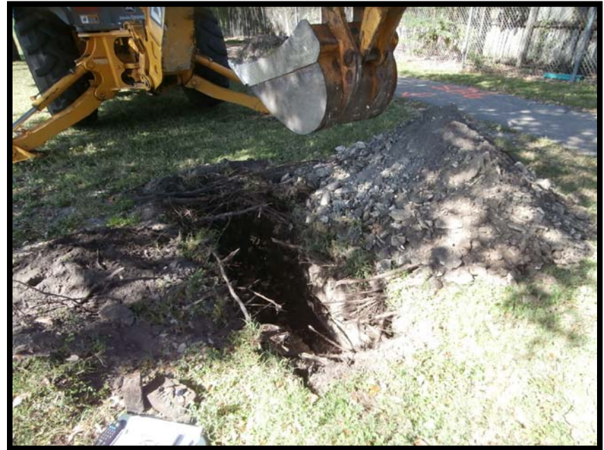
Test Pit 6. C+D debris.
