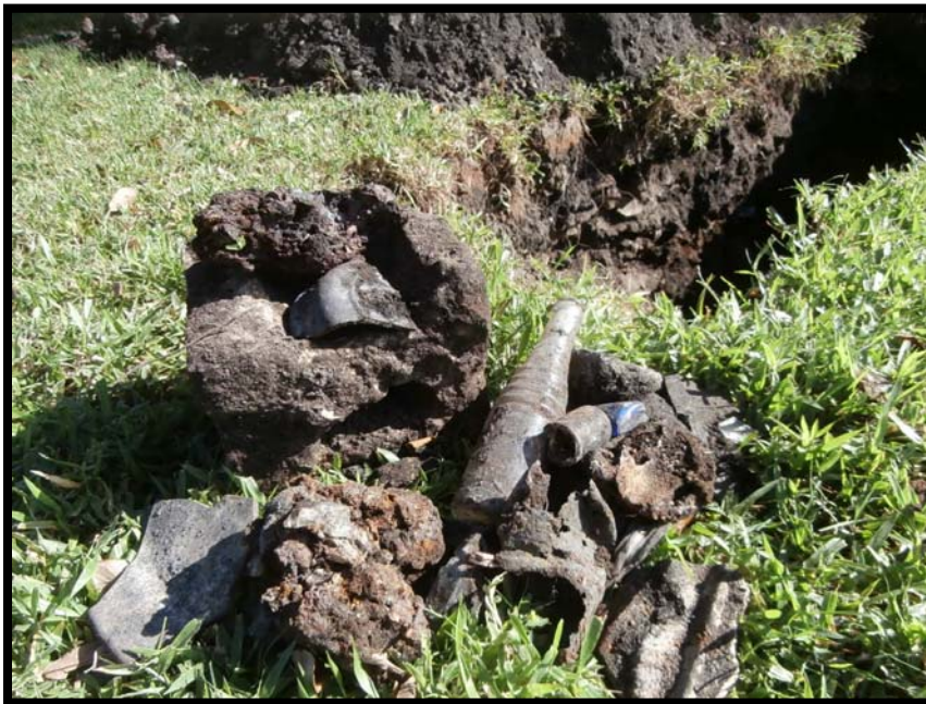
Test Pit 8. Mixed solid waste debris.
