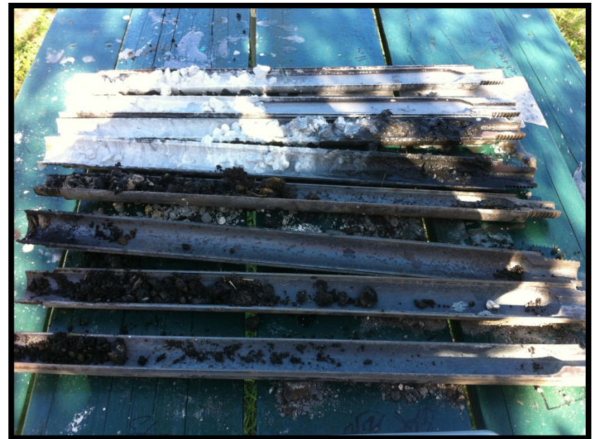
SB 16. Native limestone (stained gray) in contact with possible incinerator residue.
