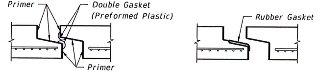
Filter Fabric Jacket Required PREFORMED PLASTIC JOINT (BEFORE PULL-UP) Filter Fabric Jacket Required PROFILE RUBBER GASKET (BEFORE PULL-UP)
