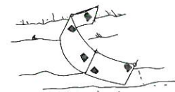
Type III Silt Fence
