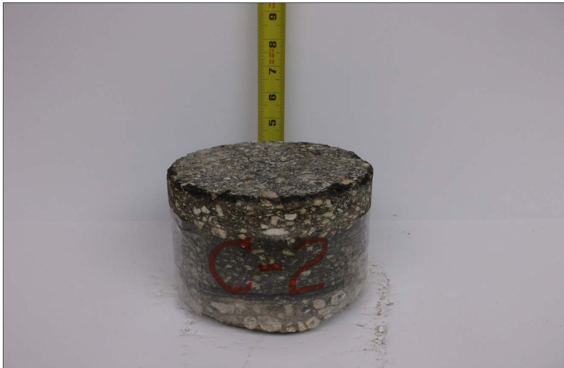
Asphalt Core No. C-2 Core Thickness 4.0 in.
