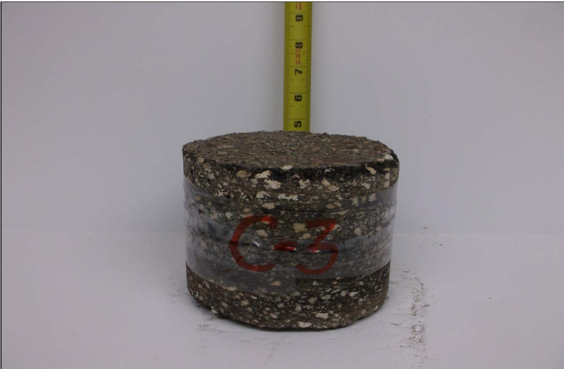
Asphalt Core No. C-3 Core Thickness 4.5 in.
