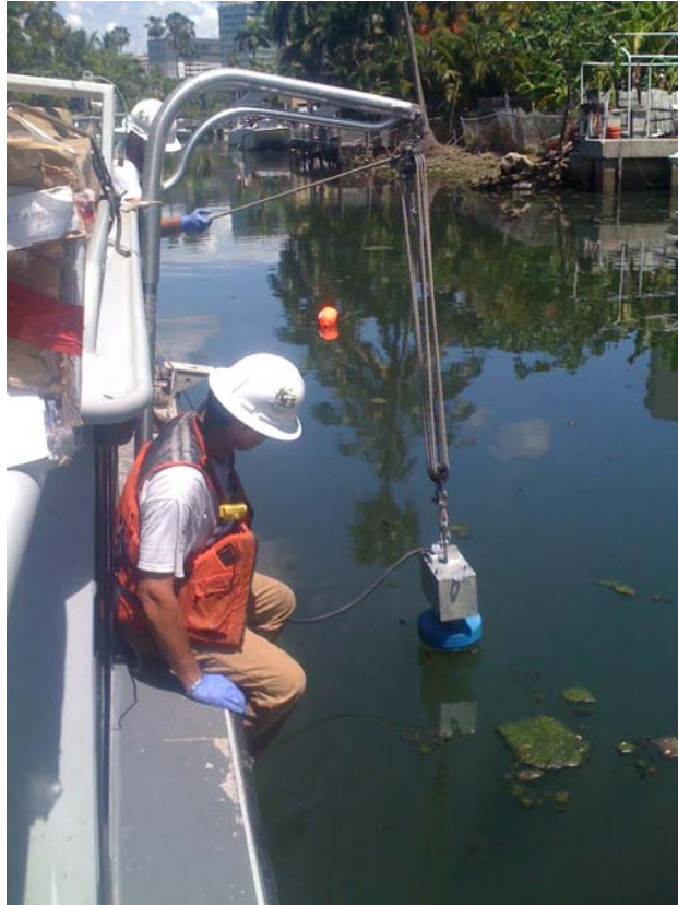
Vibecore advancing into sediment at location CH-41 within Seybold Canal.
