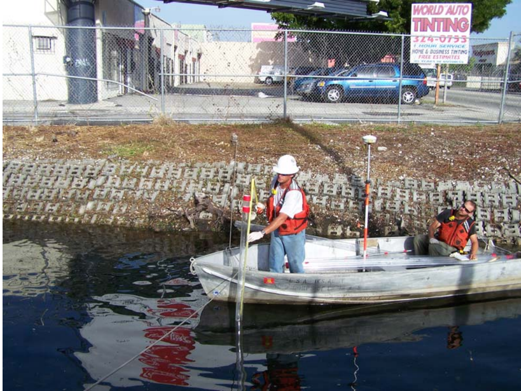
Measuring sample core depth within Wagner Creek at transect CH-1.
