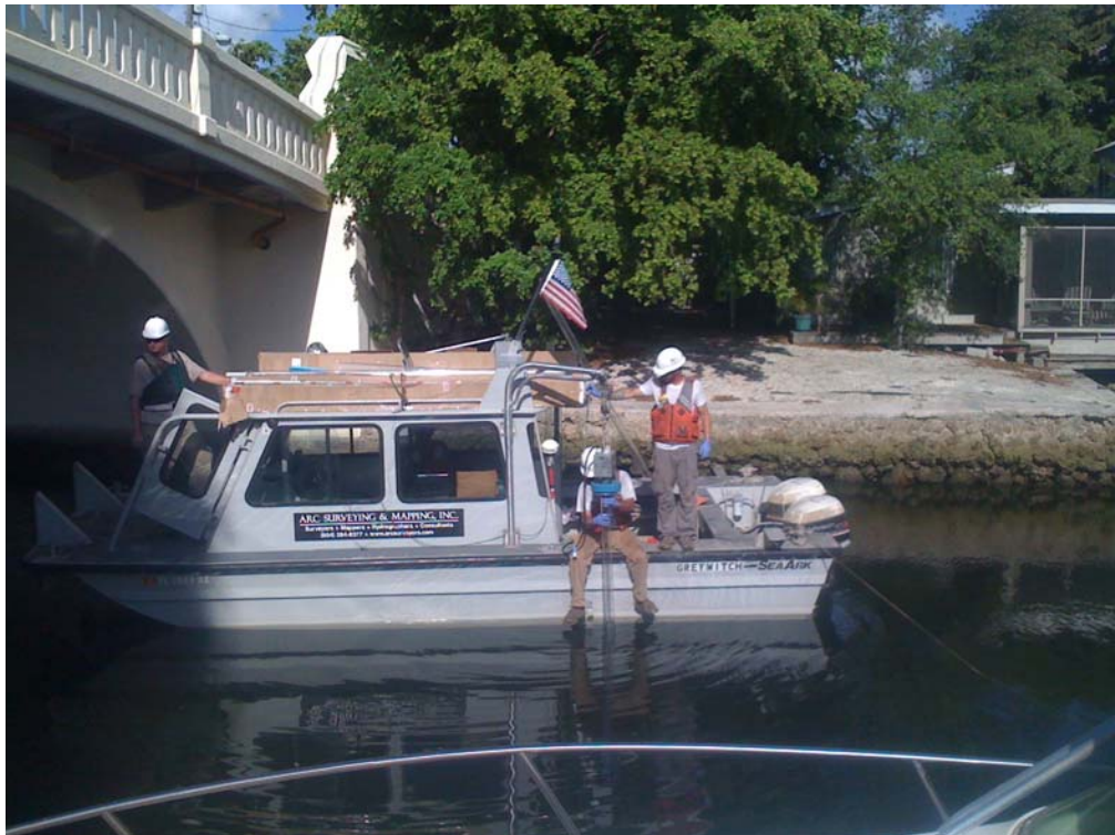
Collecting sediment sample with Vibecore within Seybold Canal at location CH-41.
