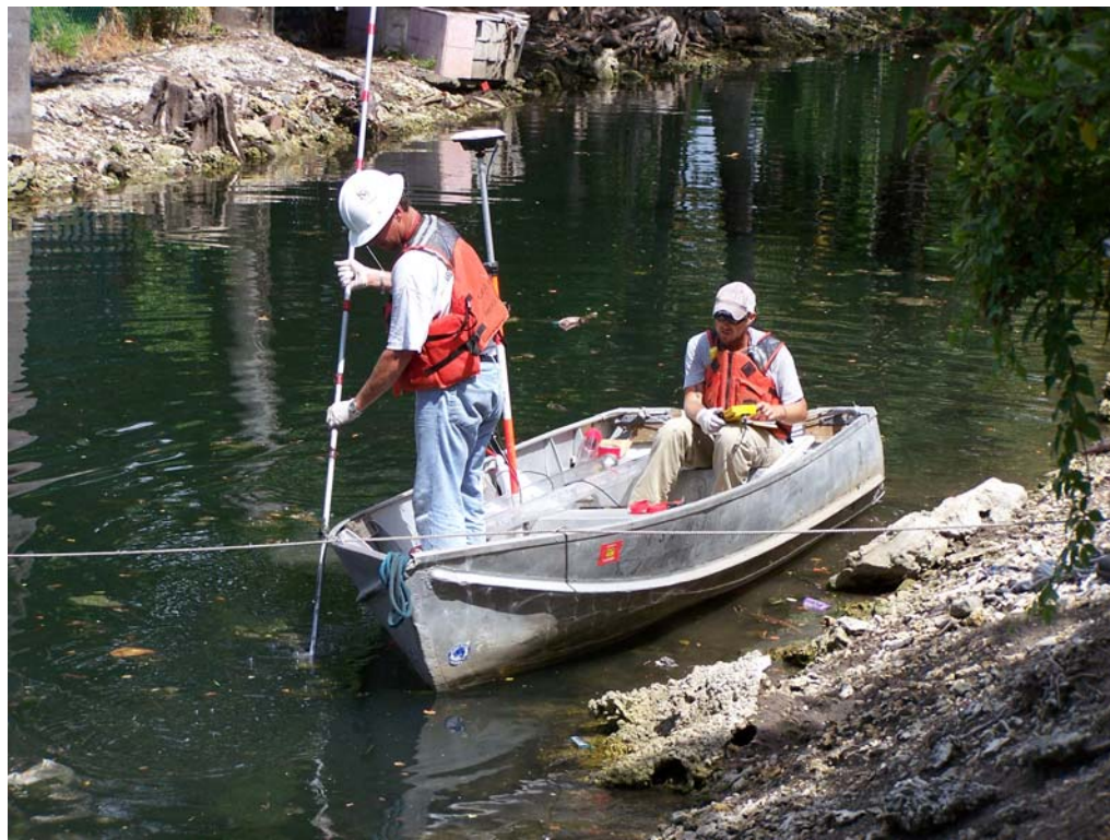
Advancing the probe rod to determine sediment thickness within Wagner Creek at transect CH-14.
