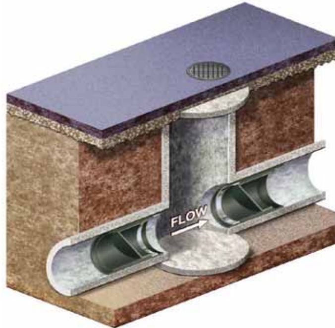
Figure 5.2.1 – Typical in-line back-flow preventer installation
