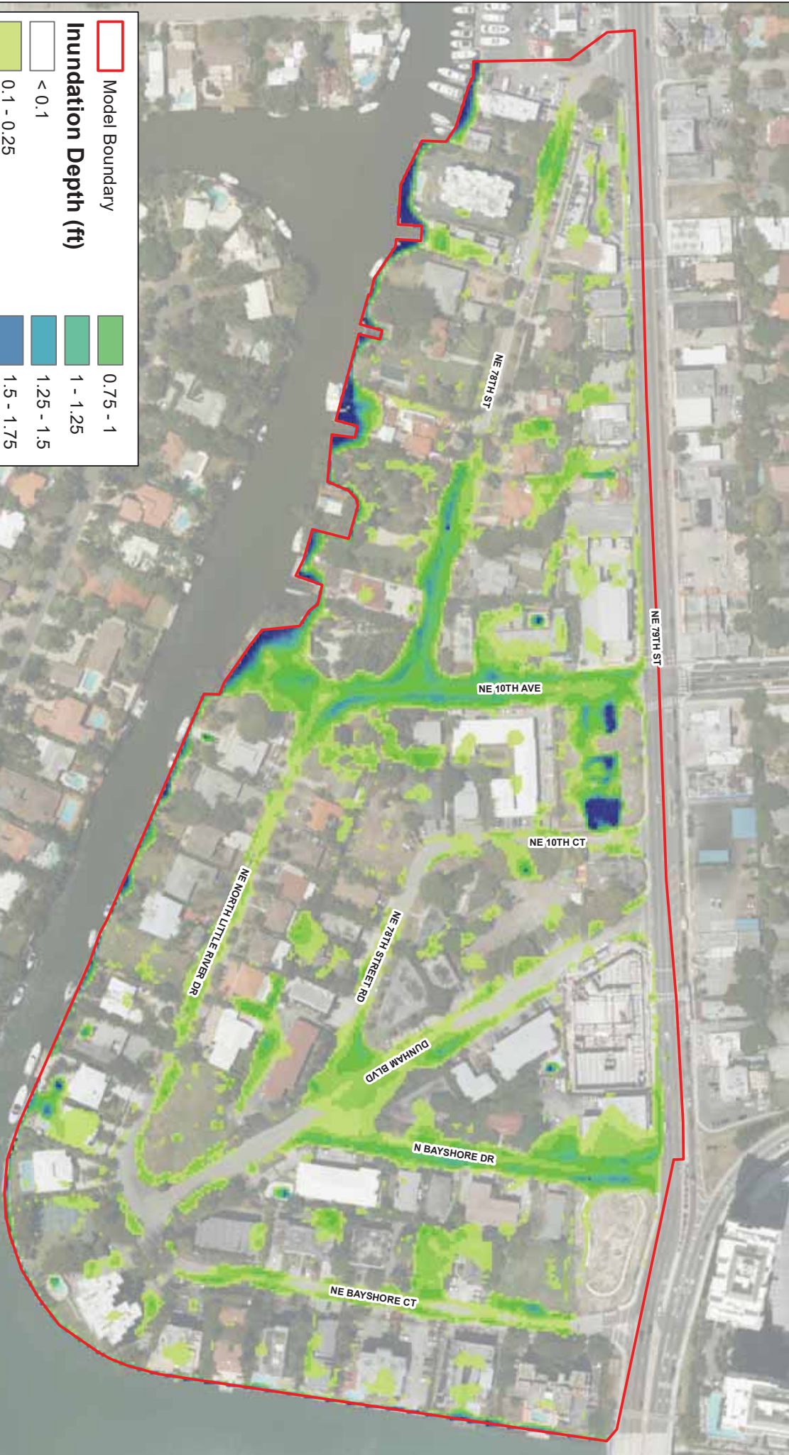
Shore Crest Drainage Feasibility Study TM 2 - Existing Conditions Assessment 5-Year, 1-Day Inundation Map
