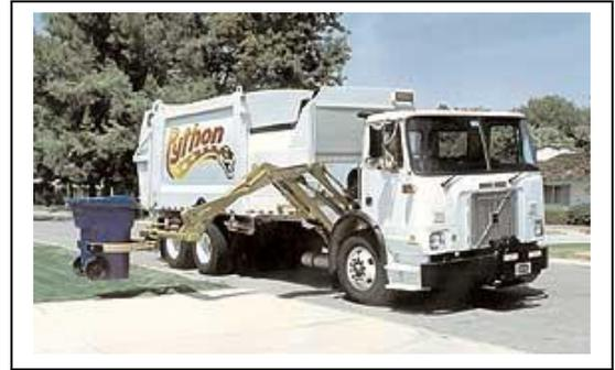
Disengage PTO or Pump Switch when Refuse Unit is not in use, being repaired or worked upon or when traveling for longer than 2 minutes.
