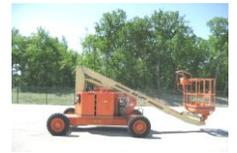
5. Prior to use, the equipment shall be given a warm up period. The hydraulic system and the lift controls shall be checked and tested daily before use to determine such features are in safe working condition. Malfunctions or unsafe operational conditions shall be reported to the foreman. Equipment, which is not in proper operational condition, shall not be used.
