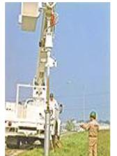
7. The truck shall not be moved unless the boom is lowered, the bucket cradled and secured, and the outriggers retracted.
