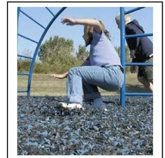
5. Make sure **spaces** that could trap children, such as openings in guardrails or between ladder rungs, measure less than 3.5 inches or more than 9 inches.
