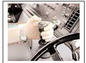
When unit is in transit to and from route, landfill, etc.; operate this vehicle from the normal driver's side.
